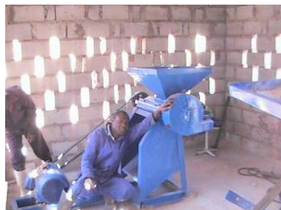
A dehuller being installed at the Milling Project next to the Carpentry Dept
